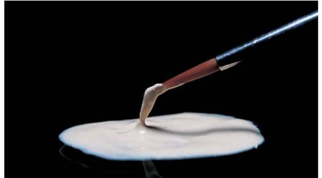
Apply a thin layer of mixed opaque with a brush or instrument and tap lightly - this will ensure close contact with the alloy.
